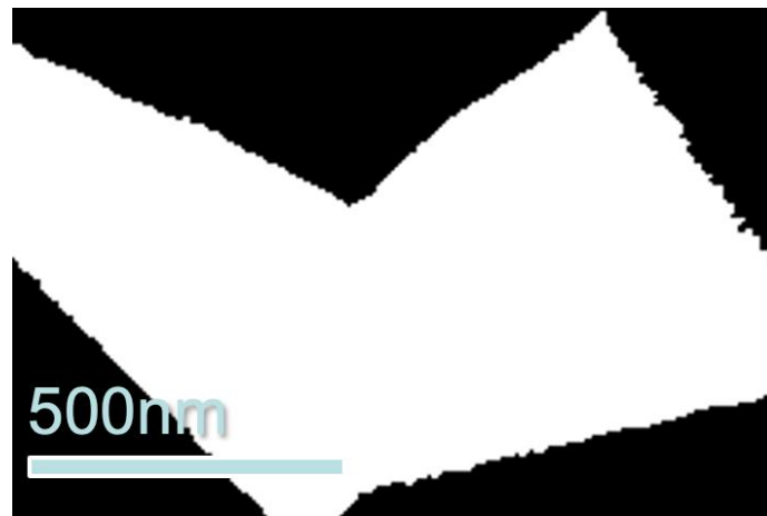
Fig. 3.9 Definition of the computation region by combining adjacent grain interiors and boundary pixels.
