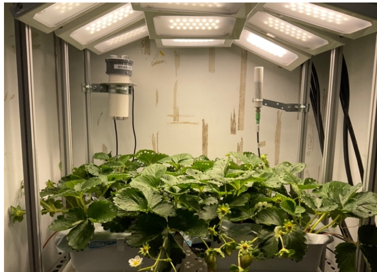
Figure 2.1 Photograph of the plant growth chamber where nine LED floodlights were installed above the strawberry plants. A temperature–humidity sensor with a forced ventilation shelter and a CO 2 sensor were also installed in the chamber.
