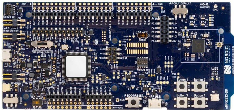
Figure 4.13: nRF52833DK board with integrated MCU unit
