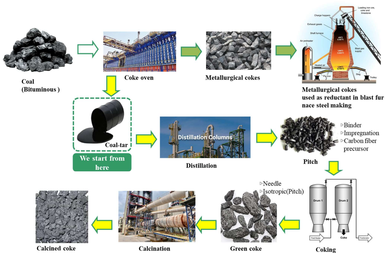
Fig. 5 Schematic of Coal /Coal-tar treatment process
