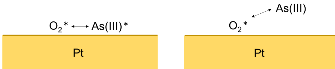
Fig. 2.9 Schematic diagram of As(III) oxidation followed by (a) the Langmuir-Hinshelwood mechanism and (b) the Eley-Rideal mechanism.
