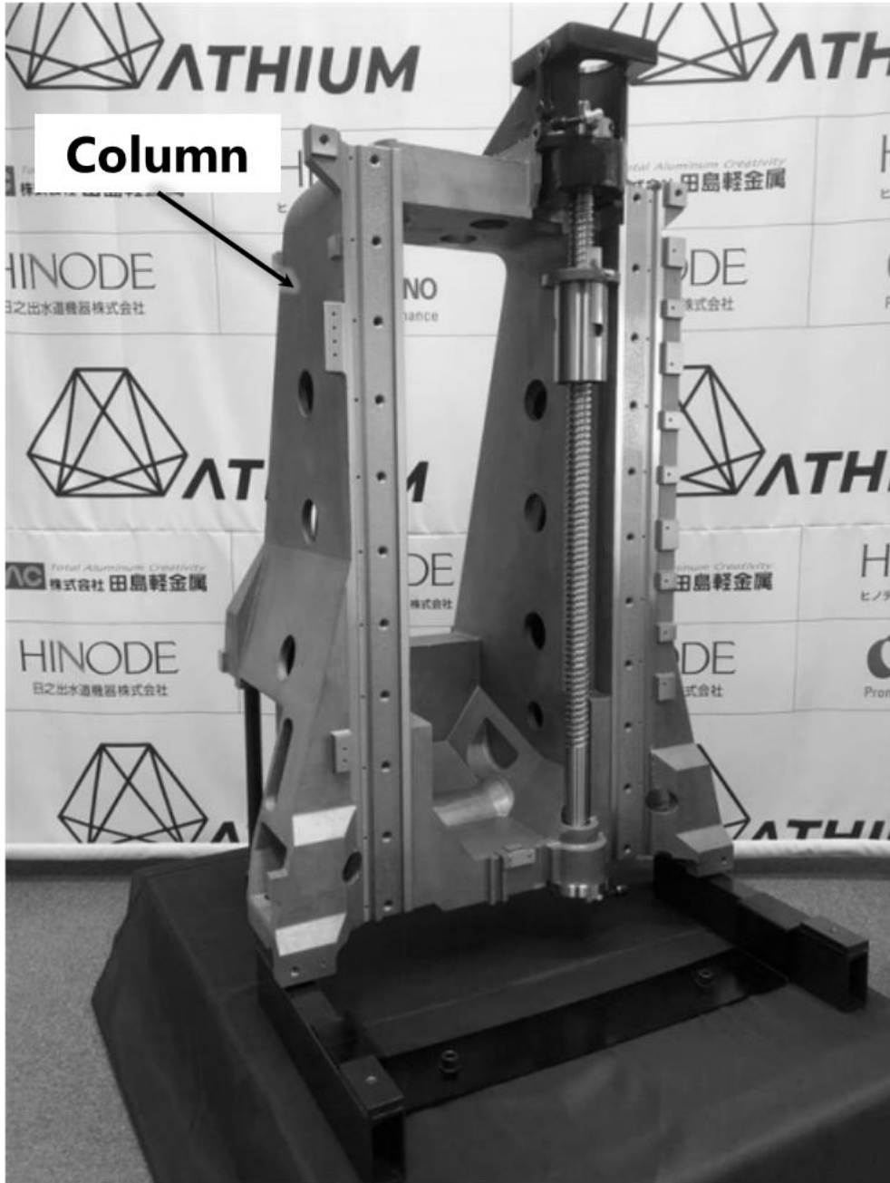
Fig.6-1 Appearance of machine tool column made from ATHIUM, high-stiffness aluminum alloy.
