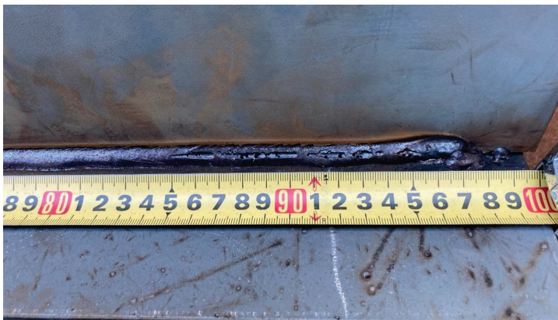
Fig. 5-9 Photograph of weld bead appearance of gas reduction
