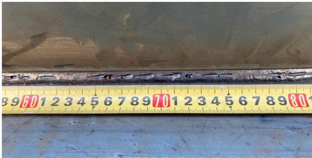
Fig. 5-8 Photograph of weld bead appearance of zinc rich primer painting
