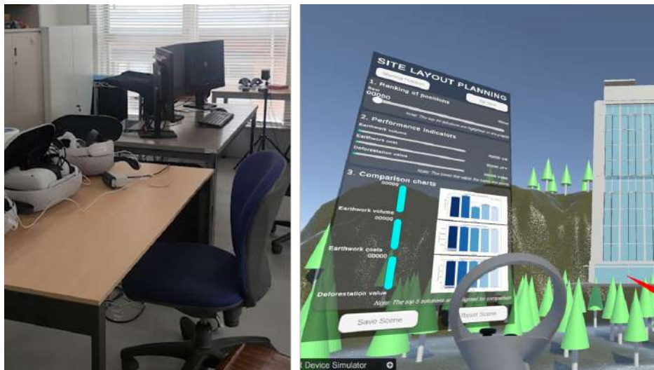
FIGURE 4.9: 'VR Interaction' stage. Detail of HUD Oculus Quest 2 (left) and Unity simulation (right).
