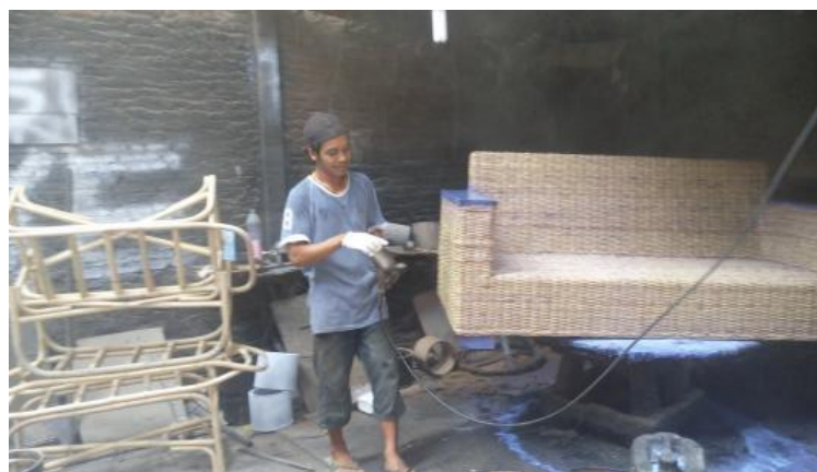
14. Finishing Sprayer (using waterbase clear coating)
