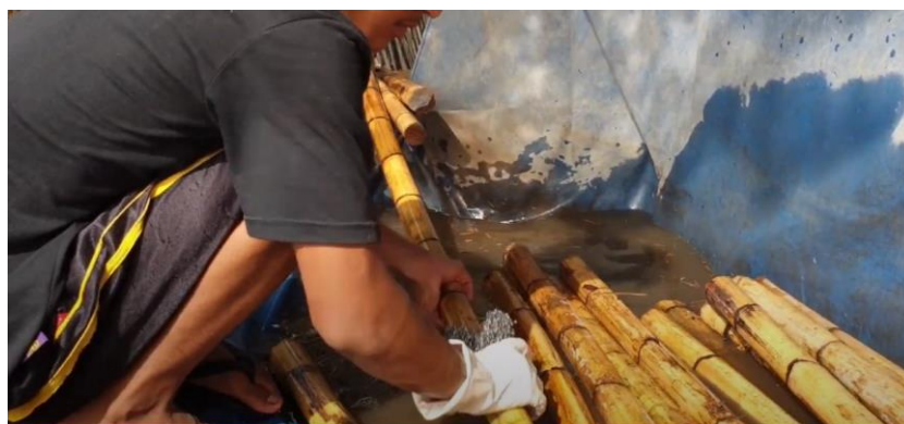
Figure 23. Rattan washing process (Source: Researcher documentation)
