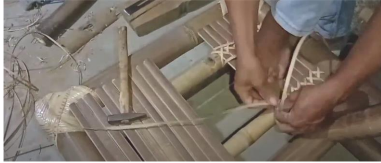
Figure 32. Binding the furniture frame with rattan (Source: Researcher documentation)
