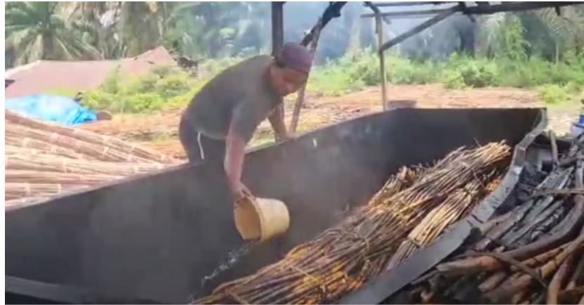
Figure 22. Rattan frying process (Source: Researcher documentation)
