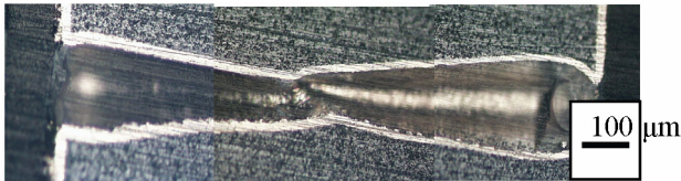
Fig. 7. Cross-sectional view of through-hole after Ni electroless plating.
