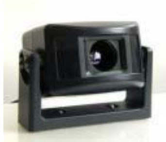
Fig. 8. Vehicle-mounted IR camera incorporated 48 x 32 element FPA
