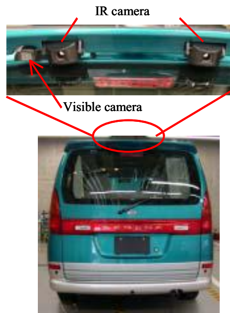
Fig. 14. In-vehicle installation of IR-RC system
