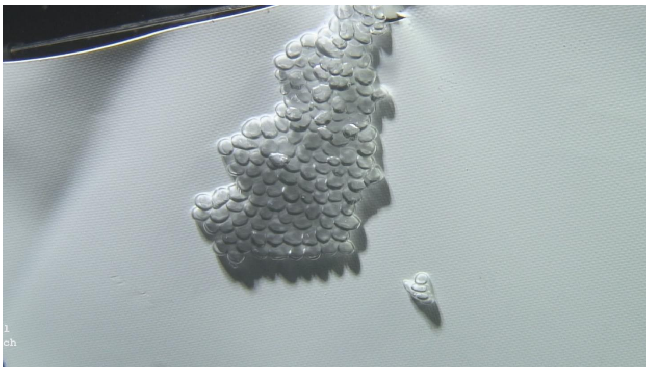
Fig. 13 MH particles accumulated on the membrane surface
