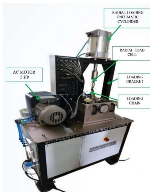
Fig. 3: Test rig of conical journal bearing.
