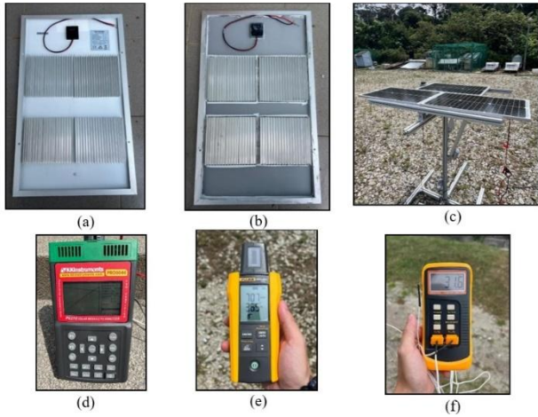
Fig. 5: (a) PV module with heat sinks, (b) PV module with heat sinks and radiative paint coating, (c) PV modules installed on DAST, (d) solar module PV analyzer, (e) Fluke-IRR1- SOL solar irradiance meter, (f) K-Type Thermometer.
