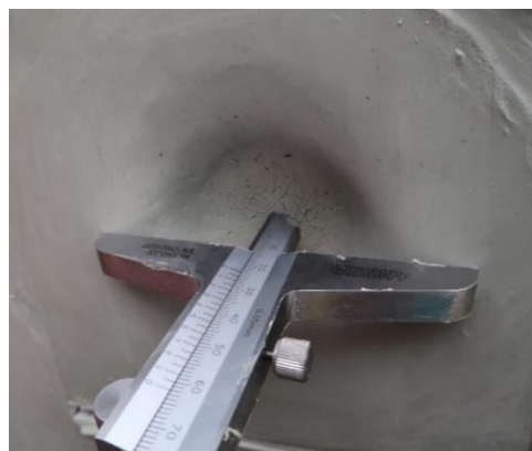
Fig. 4: Measurement of BFS on clay witnesses.
