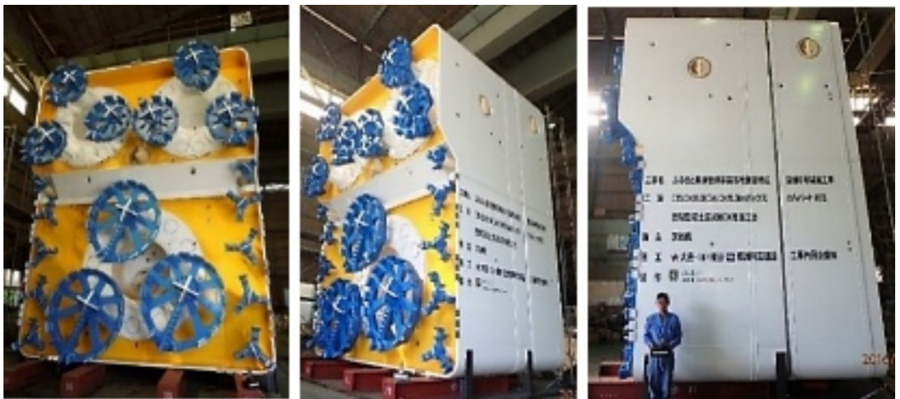
Fig. 11. Diagrams of the new RTBM developed in this project.
