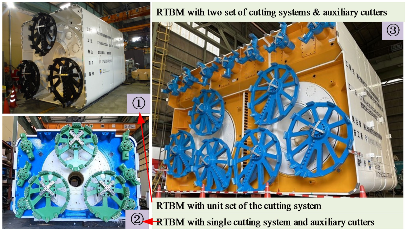
Fig. 5. Schematic diagrams of the planetary transmission mechanism-based RTBM.
