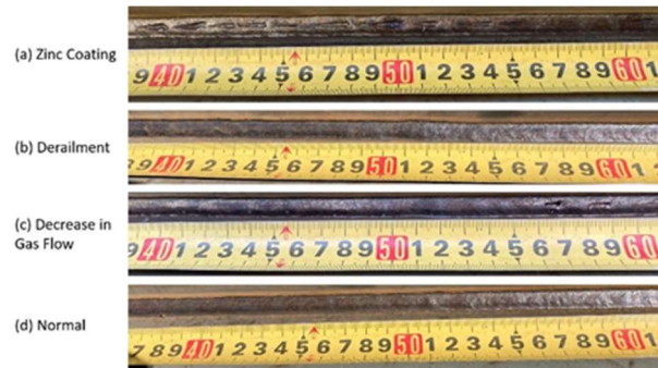
Figure 10. Weld bead appearances for each condition.
