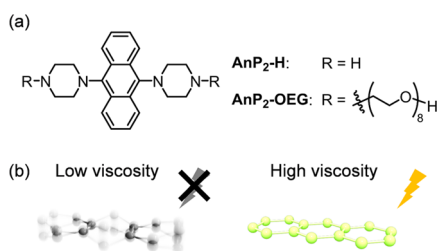
Figure 1. (a) Molecular structures of AnP 2 -H and AnP 2 -OEG . OEG denotes octa(ethylene glycol). (b) Schematic illustration of the anthracene unit after excitation at low and high viscosities.
