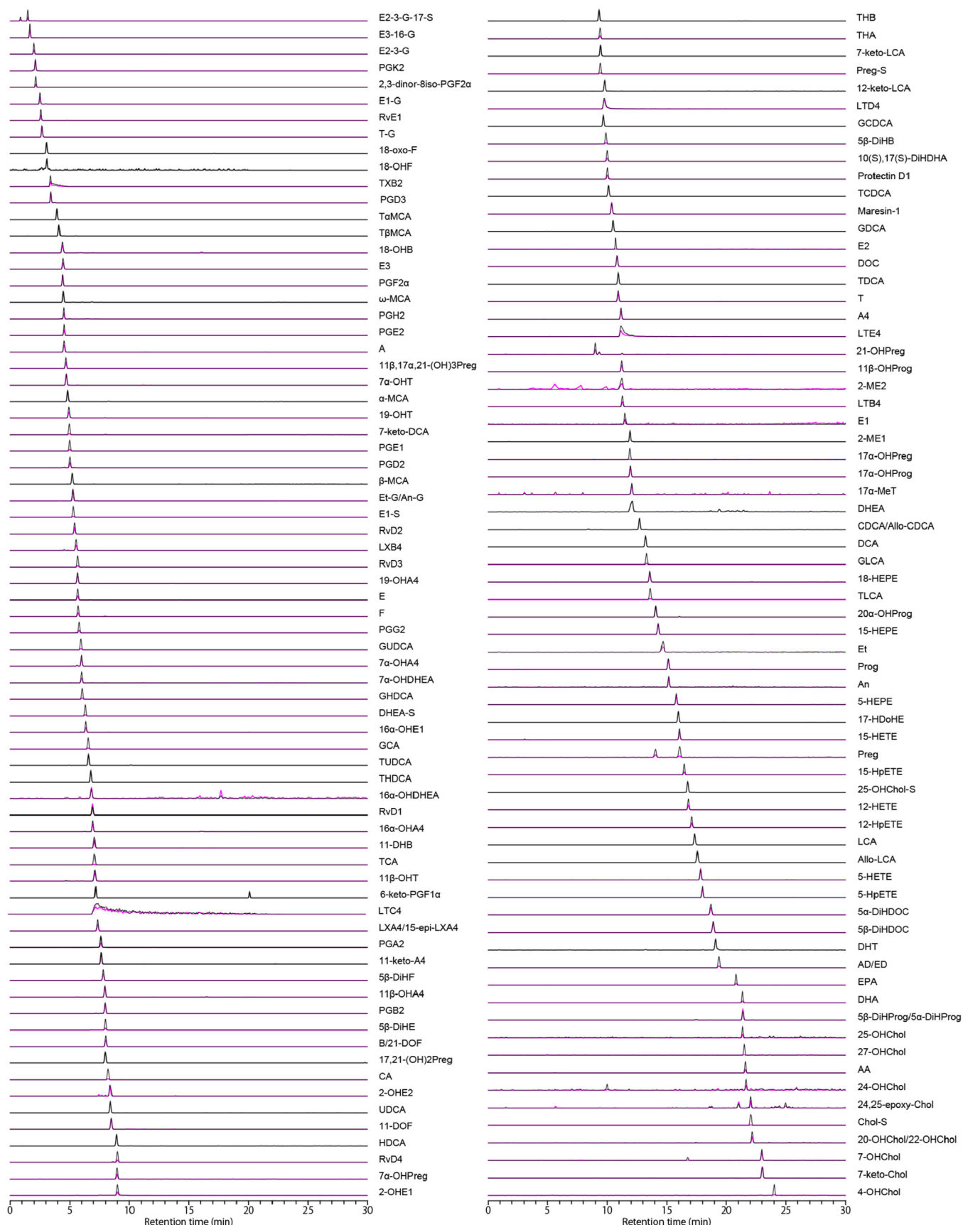
Fig. 2. Separation overview of an optimized LC/MS/MS method. Black chromatograms represent MRM/SIM transition 1 for quantification, whereas the chromatograms in pink represent MRM transition 2 for qualification. All compound abbreviations and MRM/SIM conditions are listed in supplemental Table S5 . MRM, multiple reaction monitoring; SIM, selected ion monitoring.
