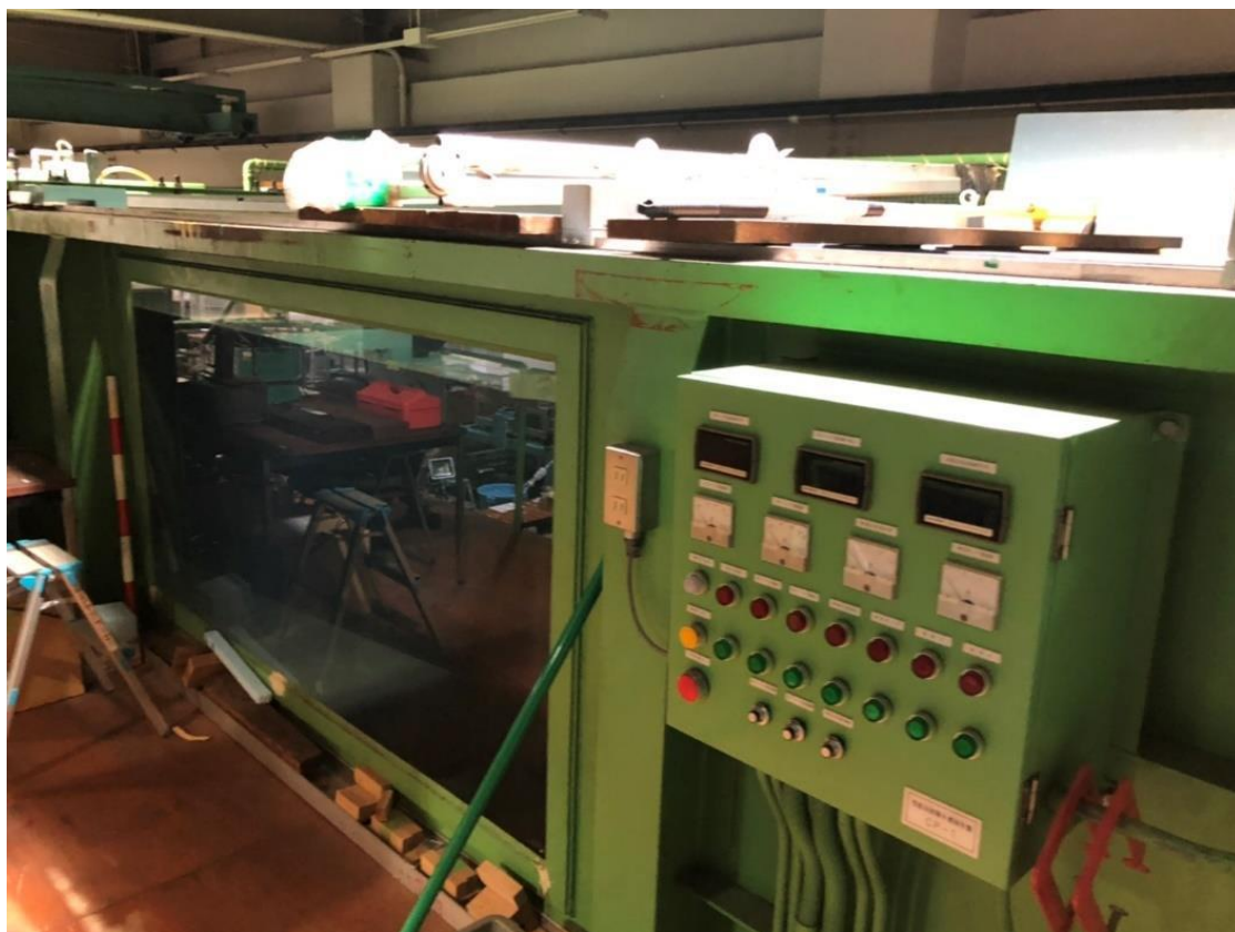
Fig.3-6 Circulating water tank at the Research Institute for Applied Mechanics (RIAM) of Kyushu University.
