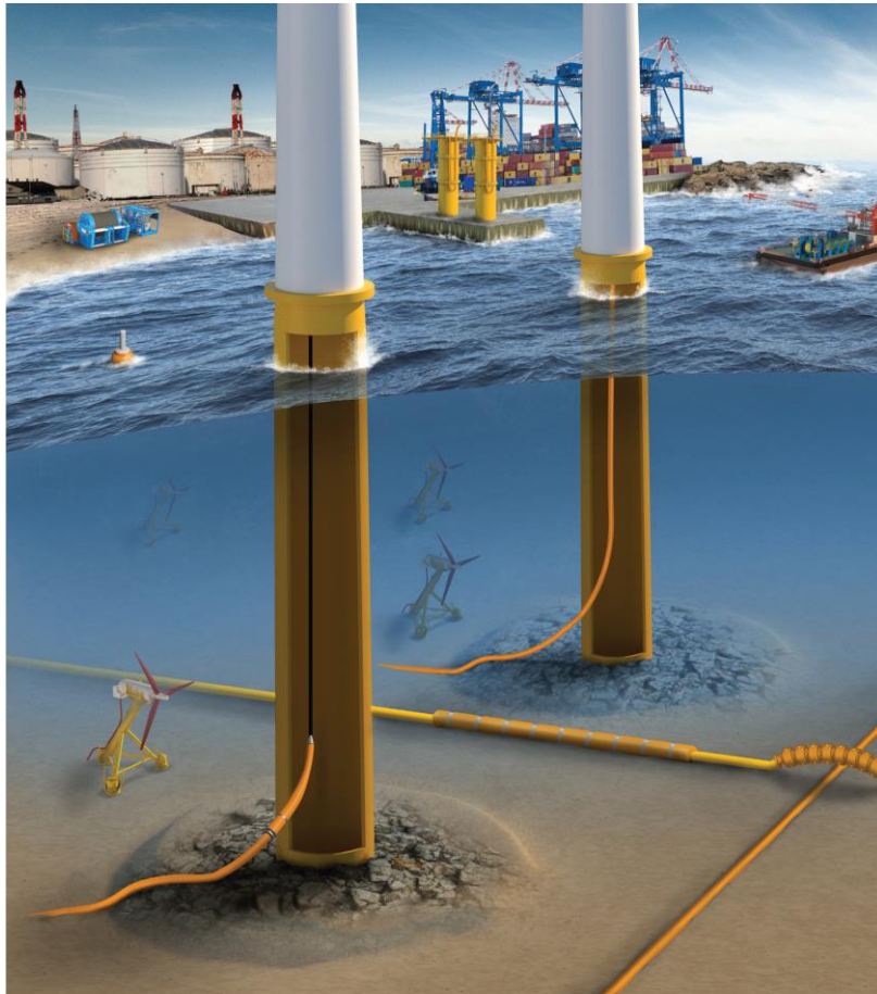
Fig.1-8 Submarine cable of the offshore wind farm [32].
