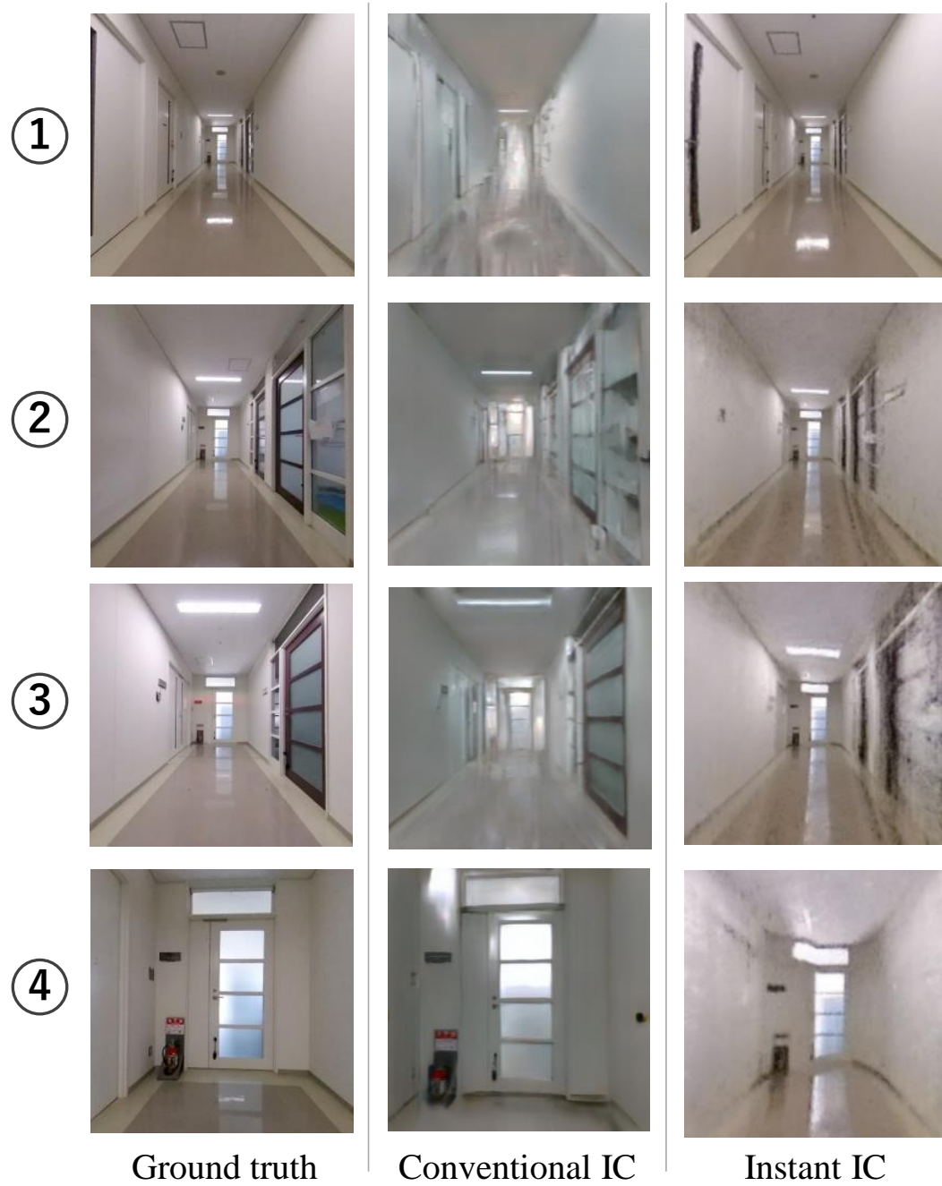
Figure 3.5: Qualitative results of the reconstruction accuracy. In conventional IC [2], the v -space is constructed by 3D scanner (FARO Focus3D [8]). ①–④ show time-series changes, with the younger numbers indicating earlier times.
