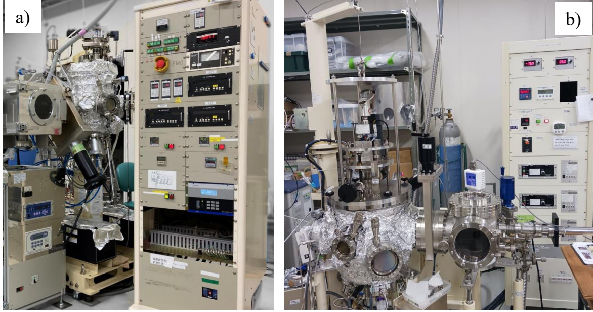
Figure 2.2 Photograph of RF magnetron sputtering systems. a). for ZnO:Co film and b). for TmIG films.
