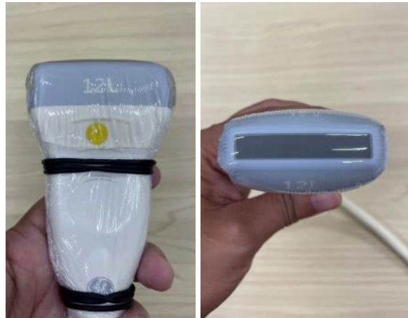
Figure 3.1 Hydrogel pad attached to the transducer.
