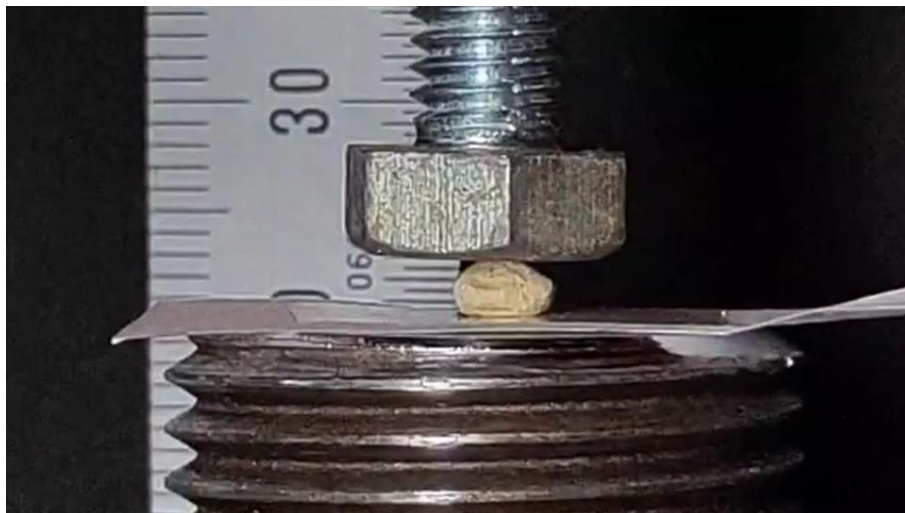
Figure 4.3 Single-particle strength test
