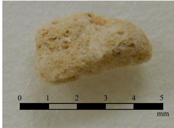
Figure 4.1 Single pumice particle for single-particle strength test
