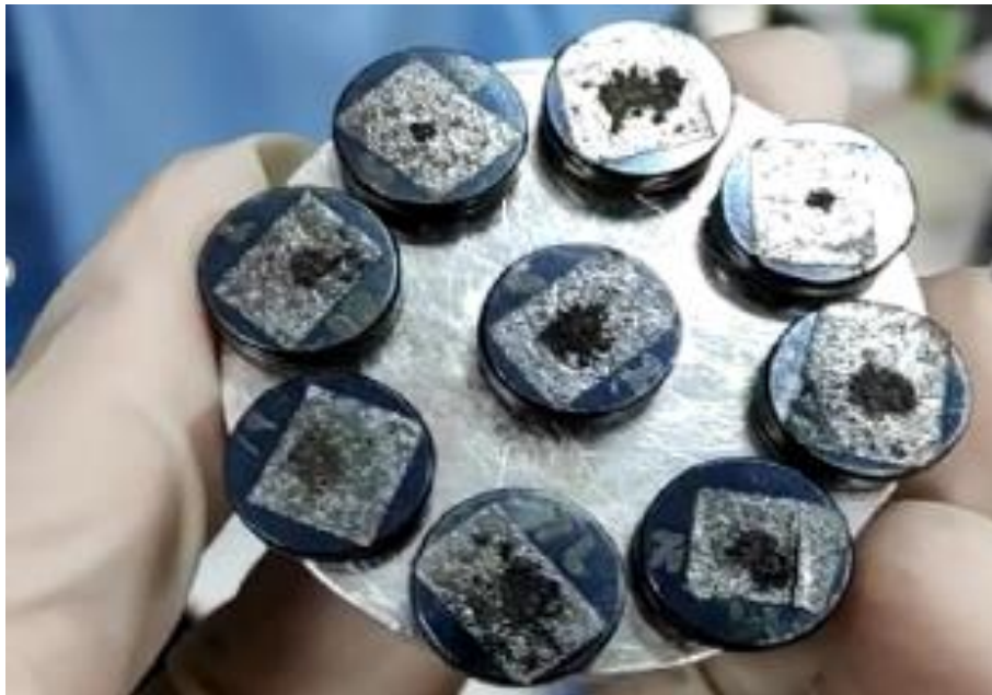
Figure 3.9. SEM and EDS sample after coating
