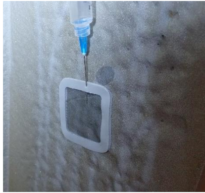
Figure 6-3 Assessment of surface salinity levels following AWT processing using the Bresle patch method.
