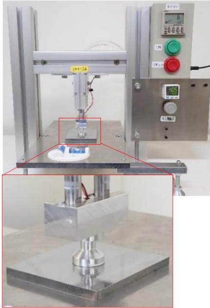
Figure 3-2 Pressurization device and dolly compression process. Figure 3-3 Desktop pull-off adhesion tester.
