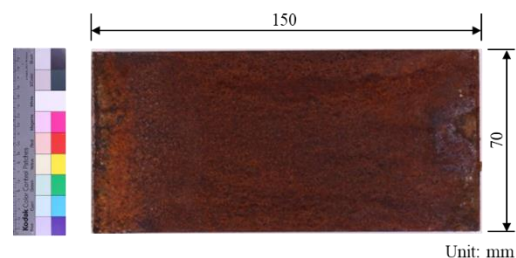
Figure 5-4 Appearance of corroded carbon steel plate.
