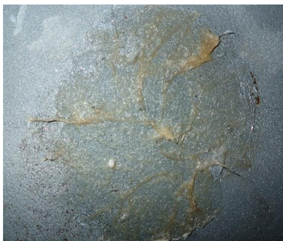
Figure 5- 6 The weak adhesion of cotton-like fibers to the steel surface after SACP tests.
