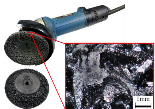
Fig. 2-2 Photographs of five kinds of surface treatment tools
