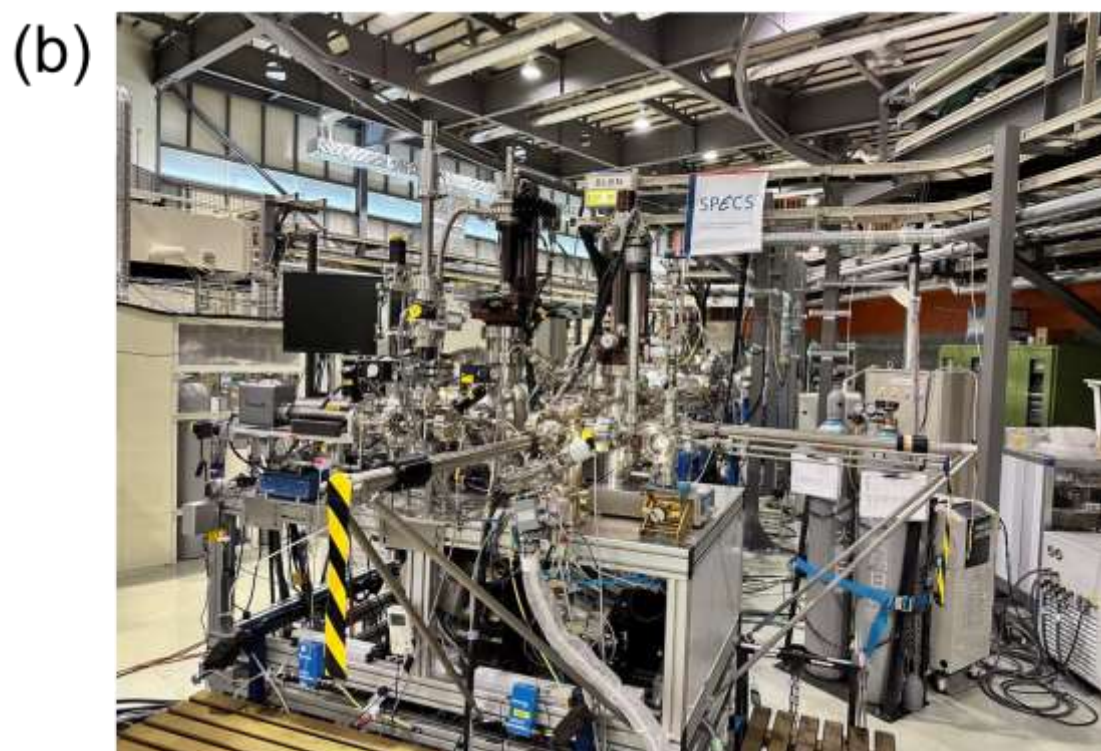
Figure 2.19. Photos of the XAFS stations at (a) BL22XU at the SPring-8 and (b) BL6N1 at the Aichi SR.
