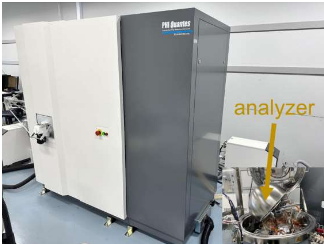
Figure 2.10. Photo of apparatus for XPS. The inset shows the electron analyzer inside the chamber.
