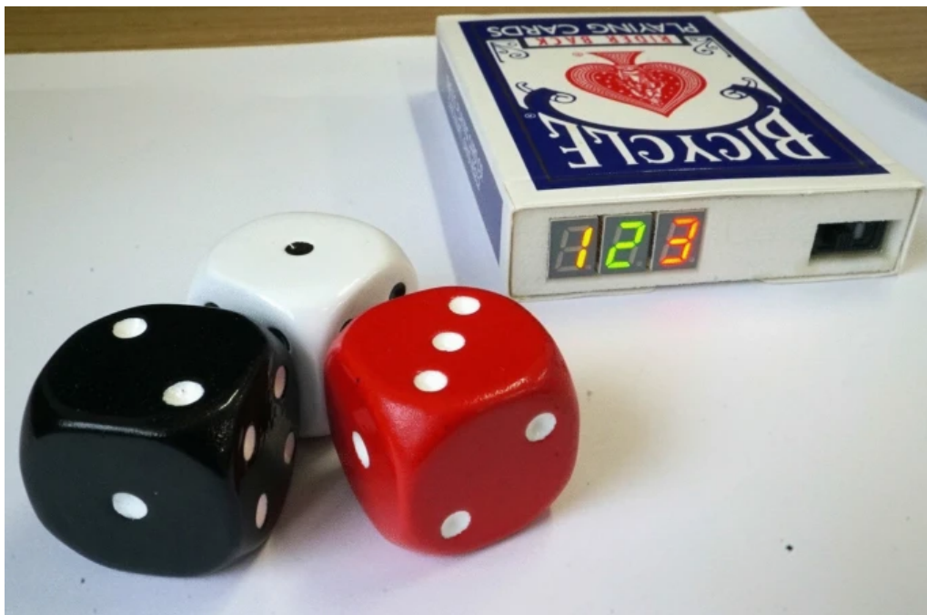
Figure 1.3 Mental Dice, numbers on the dice correspond to numbers on the remote controller
