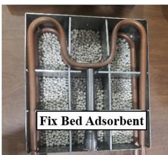
Fig. 3: Fix bed adsorbent with aluminum plate and thermowell located inside the bed duct.
