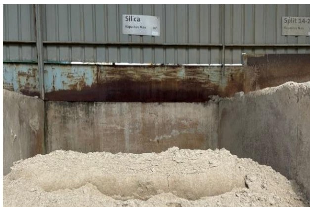
Fig. 1: Silica sand fine aggregate (0.0 – 5.0 mm).
