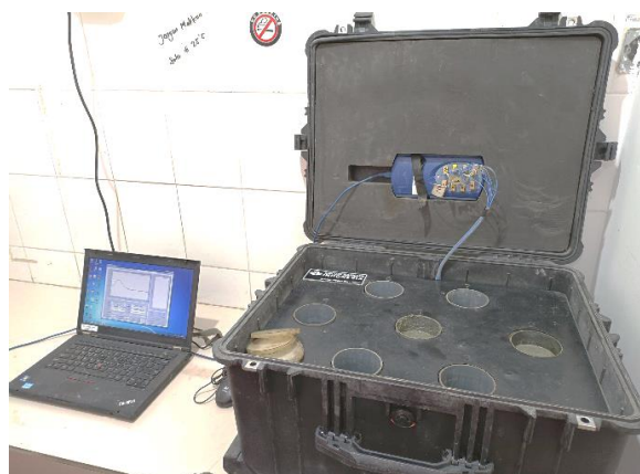
(b) Apparatus for setting time measurement. Fig. 8: Sample preparation and apparatus for the initial setting time measurement.
