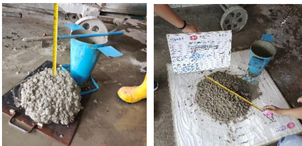
(a) Normal flow of concrete (b) High flow of concrete. Fig. 7: Slump Tests of fresh concrete.
