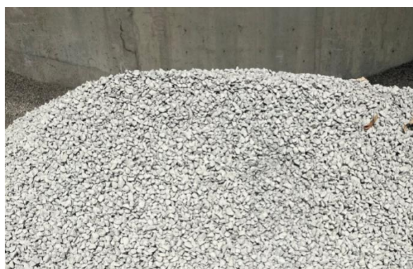
Fig. 3: The coarse aggregates (10.0 – 20.0 mm).
