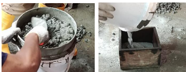
(a) Preparation of mortar sieved from concrete mixtures.
