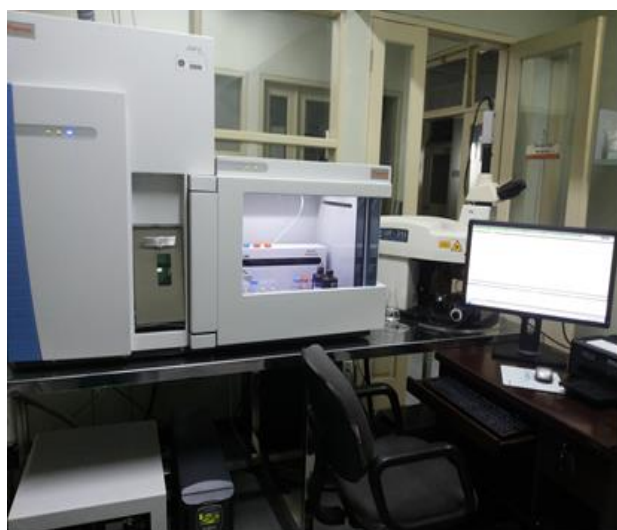
Fig. 7: ICP-MS laboratory in Centre for Geological Survey in Bandung (picture was provided by Laboratory of Geological Survey Centre in Bandung).
