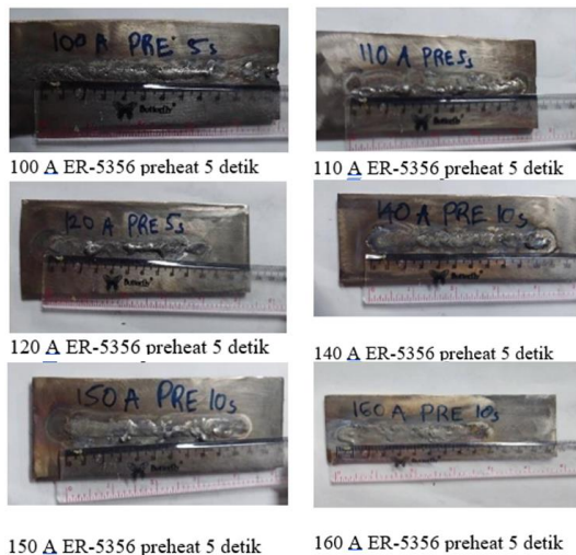
Fig. 5: TIG welding results using filler ER5356 AC polarity.
