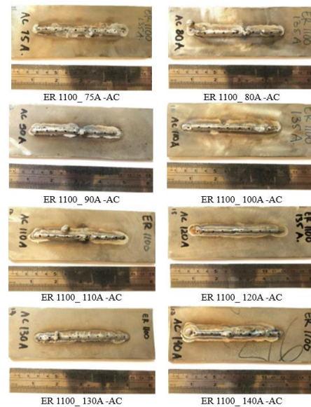
Fig. 7: Second layer welding bead (75A to 140A) filler ER1100 with AC polarity.
