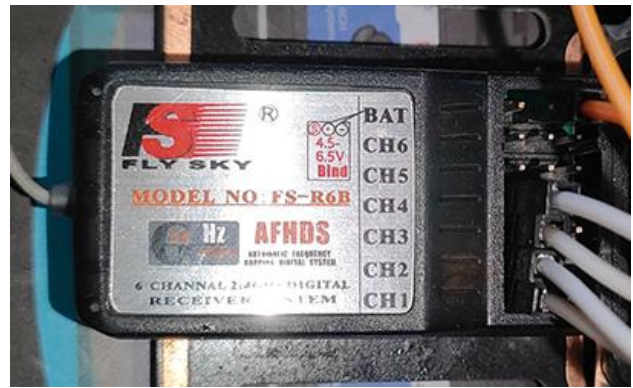
Fig. 6: RF Receiver module
