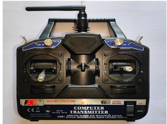
Fig. 5. RF-Remote with Transmitter module
