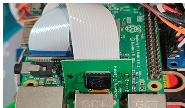
Fig. 4: Raspberry Pi with IR Surveillance Camera Module
