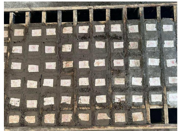
Fig. 4. Labeled and Casted Concrete Cubes
