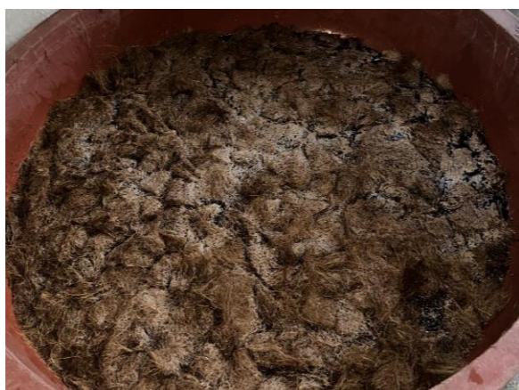
Fig. 2. Coconut Fiber soaked in NaOH Solution
