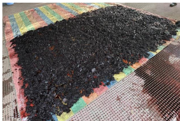
Fig. 3. Air drying of treated Coconut Shells
