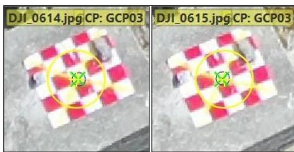
Fig 3: The process of matching coordinates and images of control points.
