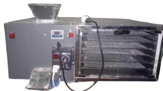
Fig. 5. Fabricated Small-Scale Integrated Saba Banana Flour Mill.
