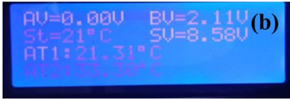
Fig. 10. Arduino supply voltage is (a) between 5V to 12V and (b) less than 5V.
