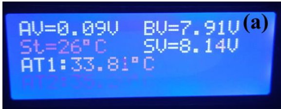
Fig. 10. Arduino supply voltage is (a) between 5V to 12V and (b) less than 5V.
