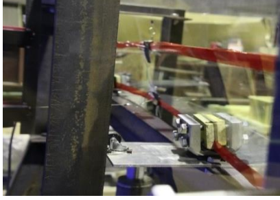
(b) Lateral-torsional buckling deformation.
