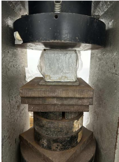
Fig. 9. Compressive strength test setup
