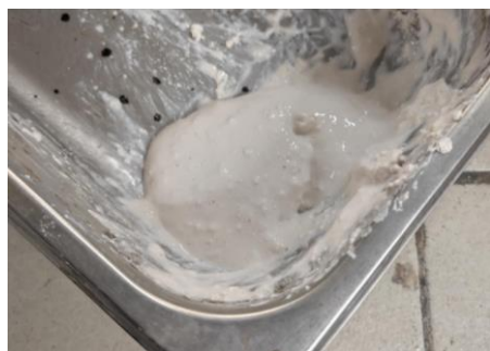
Fig. 6. Seawater-derived magnesium hydroxide protective coating slurry
