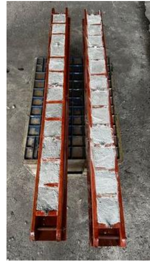
Fig. 1. Concrete placed in wooden molds
