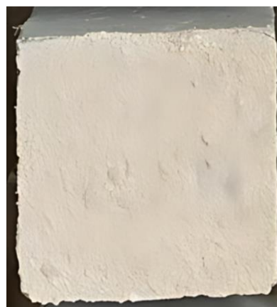
Fig. 7. Seawater-derived \text{Mg}(\text{OH})_2 coating on concrete specimen
