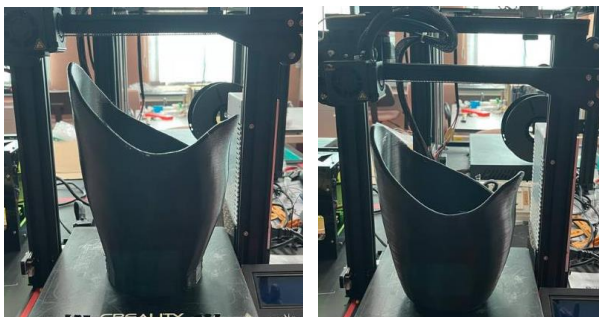
Fig. 9. Printed conventional (left) and pin-lock (right) sockets.
