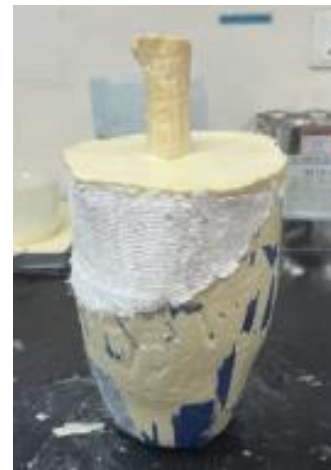
Fig. 7. Developed mock stump in conventional transfemoral prosthetic socket.
