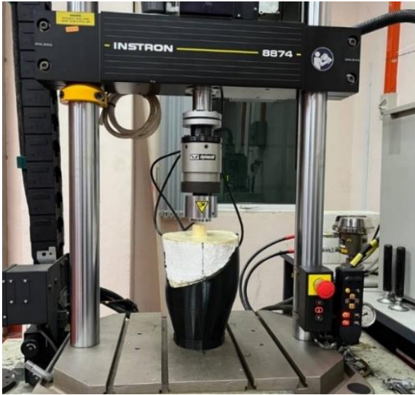
Fig. 8. Compression test setup on Instron 8874 testing machine (Illinois Tool Works Inc., Norwood, USA).
