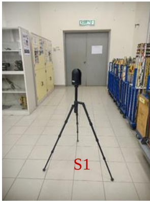
Fig. 2. Leica BLK360 laser scanner setup at Station 1
