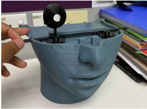
Fig. 11. Assembly of the mouth, rack gear, spur gear, and eyeball parts.
