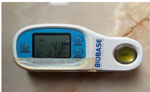
Fig. 5. Measuring TSS using sweet pepper's extracted juice
