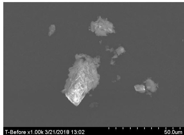
Fig. 4. SEM result of Pure Gold Mill Tailings.
