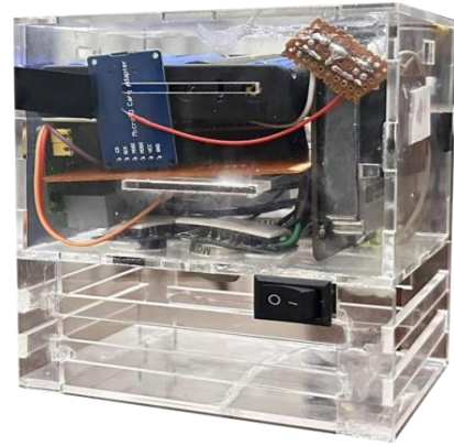
Fig. 6. IoT-Based air quality monitoring device.
