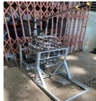
Fig. 4. Cacao-Pod Splitting Device Prototype
