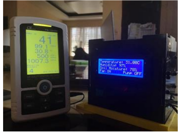
Fig. 5. DHT11 Sensor Testing
