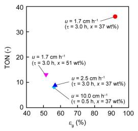
**Figure 5.** Relationship between TON and gel porosity  $(\varepsilon_g)$  of organogel monolith reactor in continuous-flow asymmetric aldol additions.
