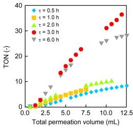
**Figure 4.** TONs of proline-supported monolith reactors at different residence time  $(\tau)$  in continuous-flow asymmetric aldol additions. Conditions: p-nitrobenzaldehyde (0.2 mol L<sup>-1</sup>, 1 eq.) and cyclohexanone (1.0 mol L<sup>-1</sup>, 5 eq.) in DMSO/ water (80:20 v/v), organogel monolith column (x = 37 wt%, L = 5.0 cm), and 30 °C.
