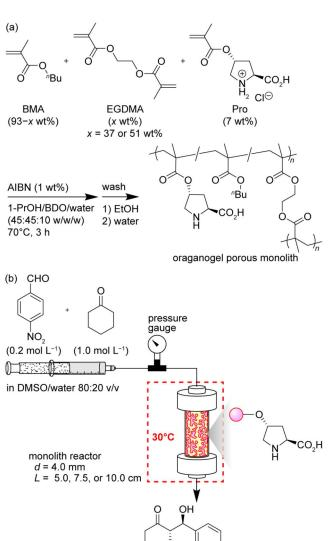
**Figure 2.** (a) Synthesis of proline supported organogel monoliths and (b) continuous-flow setup for asymmetric aldol addition between p-nitrobenzaldehyde and cyclohexanone.
