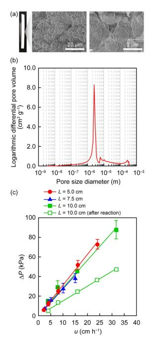
**Figure 3.** (a) Photographic (left) and FE-SEM images (center and right), (b) pore size distribution determined by MIP, and (c) continuous-flow permeability of the monolith (x = 37 wt%, measured in duplicate in two independent experiments for monoliths before flow reactions).
