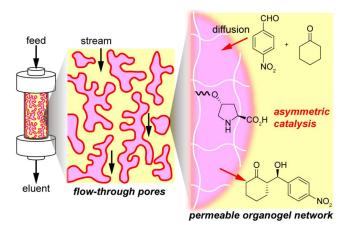
Figure 1. Schematic of organogel-based porous monolith reactor as continuous-flow immobilized catalyst.
