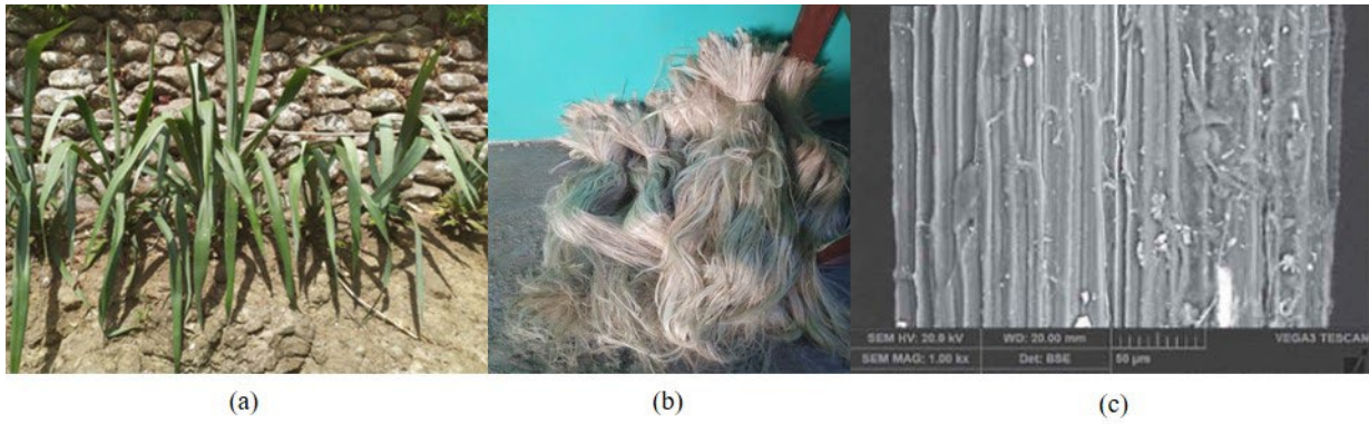
Fig.2: (a) Agave cantala plants; (b) Cantala fibers; and (c) Surface morphology of a cantala fiber observed using SEM 26)
